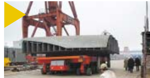
A section being transported out to the slipway. The shipyard in China constructs ships in a traditional way.
